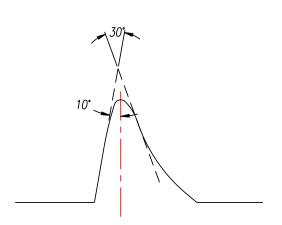
The REMFORM<sup>®</sup> II<sup>™</sup> asymmetrical Unique Radius Flank<sup>™</sup> thread form has the thread forming advantages of a 30° thread, without the difficulty of manufacturing a 30° thread.
